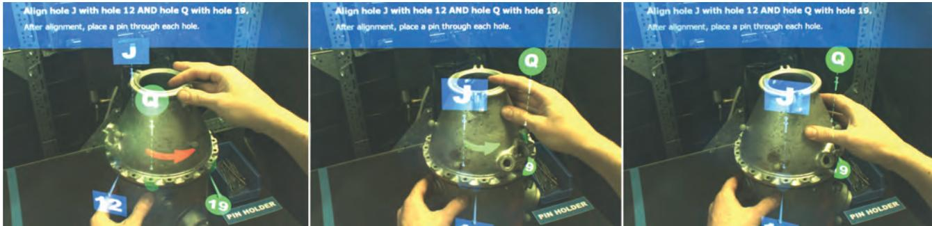
Figure 1: AR assistance for psychomotor phase of a procedural task. (Left) Dynamic 3D arrows and labels overlaid on aircraft engine components (center) respond to ongoing user activity to provide assistance in achieving (right) alignment of components. (Captured by a video camera looking through optical-see-through display used in study. A post-render filter was applied to remove camera distortion and vignetting.)
