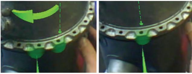
Figure 4: Dynamic highlights. (Left) Prior to alignment, distinct highlights are rendered on top and bottom holes. (Right) When holes are aligned, bottom highlight slowly fades out, presenting the appearance of a single hole. (Images show cropped enlargement of view through a video-see-through display.)
