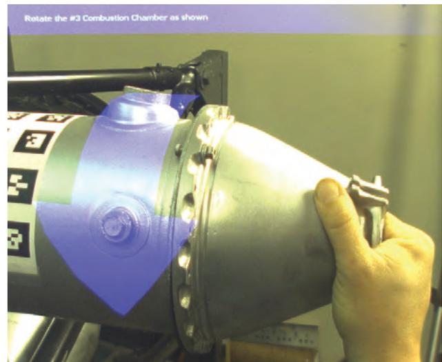
Figure 12: A different alignment task with AR assistance. (Captured by a video camera looking through the optical-see-through display. A post-render filter was applied to remove camera distortion and vignetting.)
