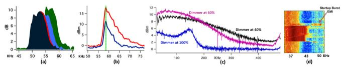
Figure 9: (a) Small, but discernable variation in the mean of the EMI peaks for four same model and brand CFLs. (b) Same CFL lamp plugged into different regions of the home producing EMI amplitude variations. (c) Band limited EMI generated by a dimmer shown at various dim levels. (d) Startup burst of EMI signal generated by CFL lamps on ignition.
