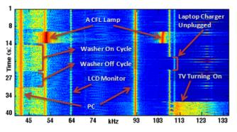
Figure 2: Frequency spectrogram showing device actuation in a home.
