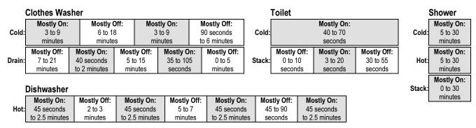
Figure 6. Clothes washer, dishwasher, and toilet activity are matched based on the mechanical patterns in their water usage. Showers are the only activity that continuously use hot and cold water while generating waste water for an extended period of time.
