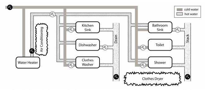
Figure 1. Schematic of the water pipes in the home where we conducted our feasibility study. The air conditioning and clothes dryer are shown because they rattled nearby pipes, introducing noise that needs to be considered in analyses. The four shaded sensors are used for modeling activities, while the unshaded sensors are included only for validating our results.
