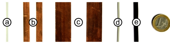
Figure 17: Cable types tested in our evaluation of sensor characteristics. A-C consist of flat copper foil traces, D and E use stranded wires.
