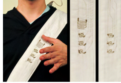
Figure 2. Top: 3 and 4-button prototypes. Bottom: 4-button multitouch interface sewn into a messenger bag strap and worn across the body.
